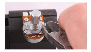
We will need to nip off the little tab on each pot. Simply take your clippers or needle nose pliers and break it off. If you are looking at the picture you would bend it to the right or away from the shaft. It is very brittle so bending it will break it off very easily. We prefer bending it.
